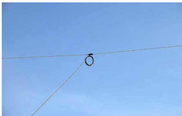
160 meter loop feed point with choke coil
