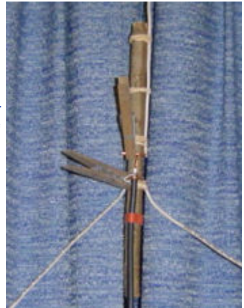
Clothes pins hold the coax center conductor to the vertical radiator and the coax shield to the two elements of the ground plane. Rubber bands hold elements and the coax in place.
